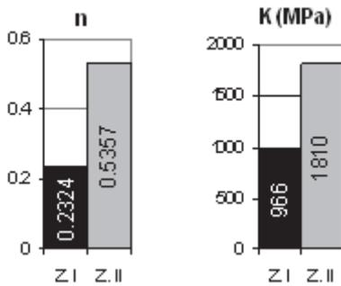
**Figure 5** Comparison of the strain-hardening parameters,  $n$  and  $K$ , for the zones I and II.
