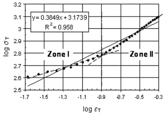
**Figure 4** Relationship between  $\log \sigma_T$  and  $\log \varepsilon_T$  (test at 18°C).
