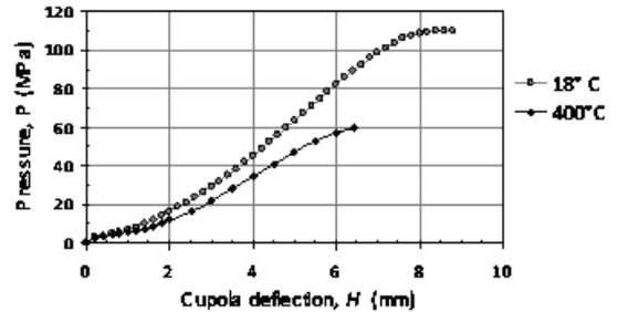
**Figure 2** Pressure-deflection curves at 18°C and 400°C.
