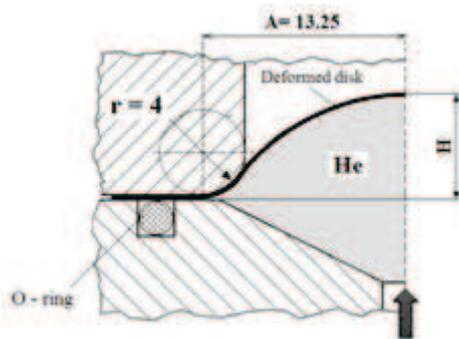
**Figure 1.** Geometry of the modified disk pressure cell
