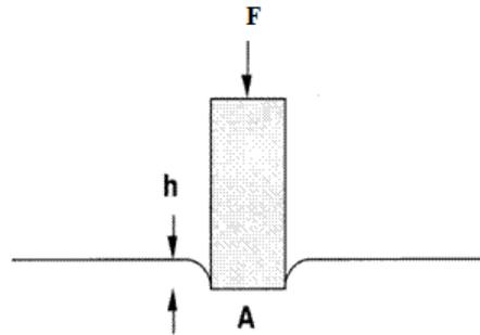
Figure 3: Schematic of the indentation creep test
