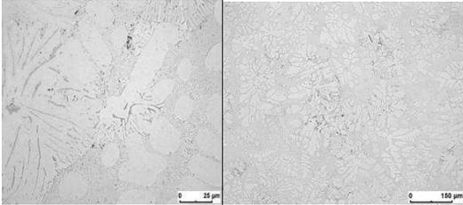
**Figure 1:** Show the microstructure of SnAg3.8Cu0,7
