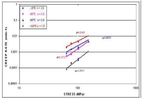
**Graph 1:** Minimum creep rate vs. applied stress at 30°C, 50°C, 80°C and 100°C
