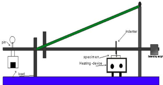
**Figure 2:** Schematic view of the construction equipment
