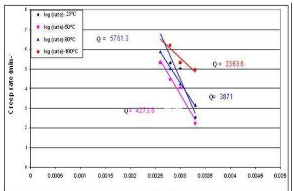
**Graph 2:** Minimum creep strain rate versus reciprocal of temperature for temperature 30°C, 50°C, 80°C, 100°C.
