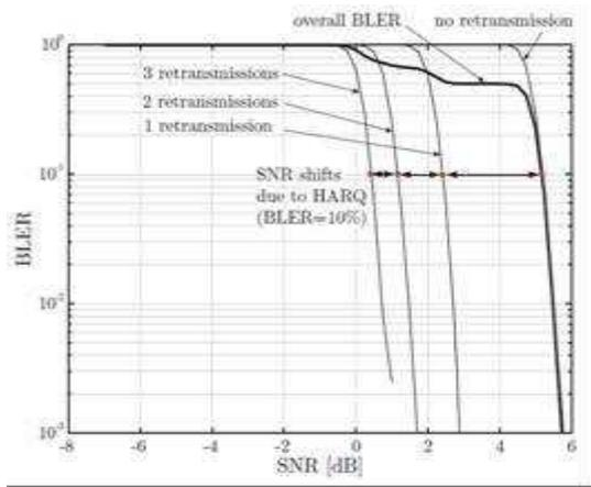
**Figure 1.** Resulting BLER at CQI=7 for different number of allowed retransmissions.
