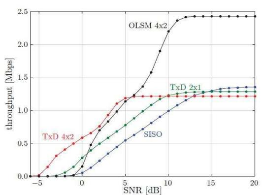
**Figure 5.** Throughput performance of the Open Loop Spatial Multiplexing (OLSM), the Transmit Diversity (TxD), the Transmit Diversity, and the SISO system over an uncorrelated ITU Pedestrian B channel (CQI 7, 3 HARQ retransmissions).
