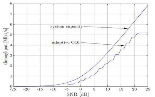
**Figure 4.** Throughput performance with AMC and HARQ over an AWGN channel
