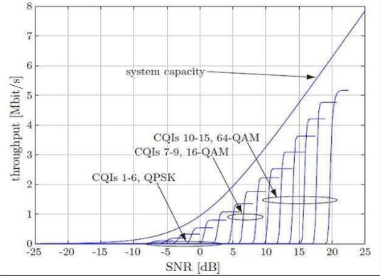
**Figure 3.** Throughput performance over an AWGN channel for individual CQIs without HARQ.
