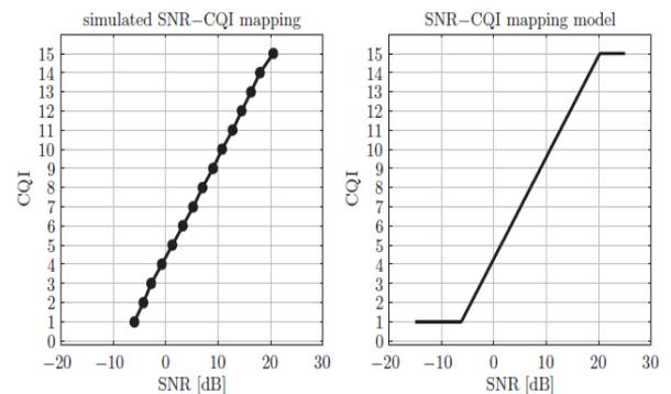
**Figure 2.** CQI mapping. BLER=10% points from the BLER curves (left) and SINR-to-CQI mapping function (right)
