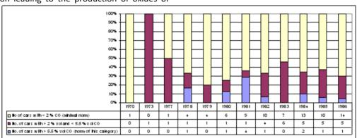
**Figure 4:** The percentage (and number) of gasoline cars produced before the year 1986, which had concentrations of CO above the norm of their category and above the minimal existing norm.
