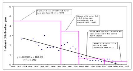
**Figure 8:** The average values of % vol CO according to production years of gasoline cars in Tirana, in comparison with the new norms for CO, in power since February 2010
