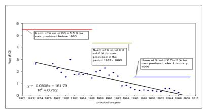
**Figure 7:** The dependence of average concentrations of CO (in % vol) from the year of production for the entire target group of gasoline cars, compared with the norms in power during the study time.
