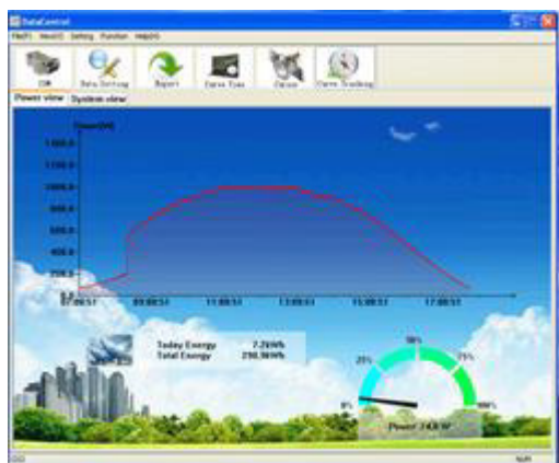
Figure 3. Daily graph of power produced by the PV Plant
