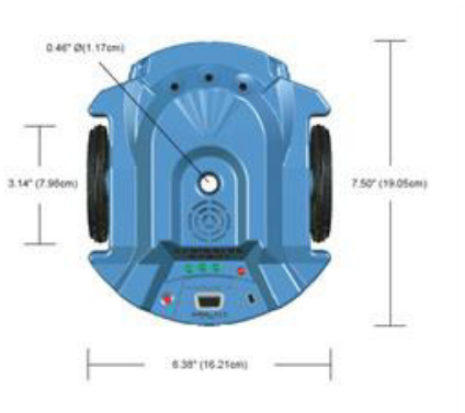
Figure 1. Scribbler S2 robot dimensions [1].
