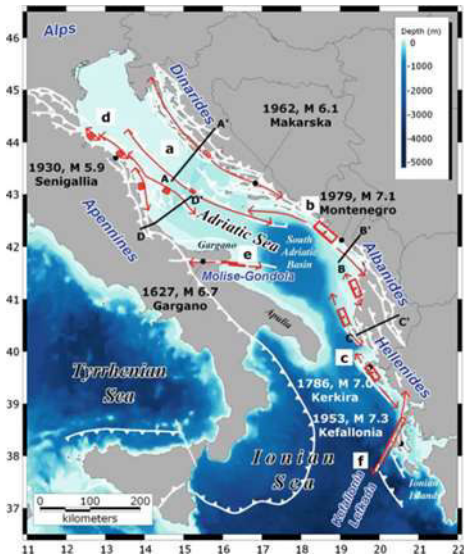
Fig.1. Tectonic sketch map of the Adriatic basin. The double-headed arrow indicates the floating path of the Typical Faults. a) Coastal and Offshore Croatia; b) Montenegro; c) Albania – Northern Greece; d) Northern Apennines; e) Apulia; f) Kefallonia-Lefkada.
